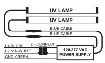
"DT" & "NEMA-R3" line-voltage dual lamp wiring
